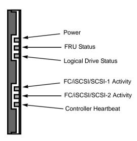
Figure 2. VTrak M300f/i/p and M200f/i/p front panel LED display
